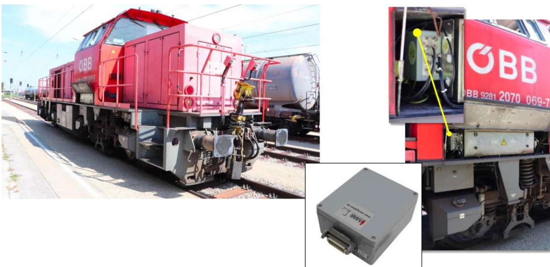
Figure 5: iRailLoc-C (localisation (INS/GNSS/ODO/+)) on shunting locomotive
