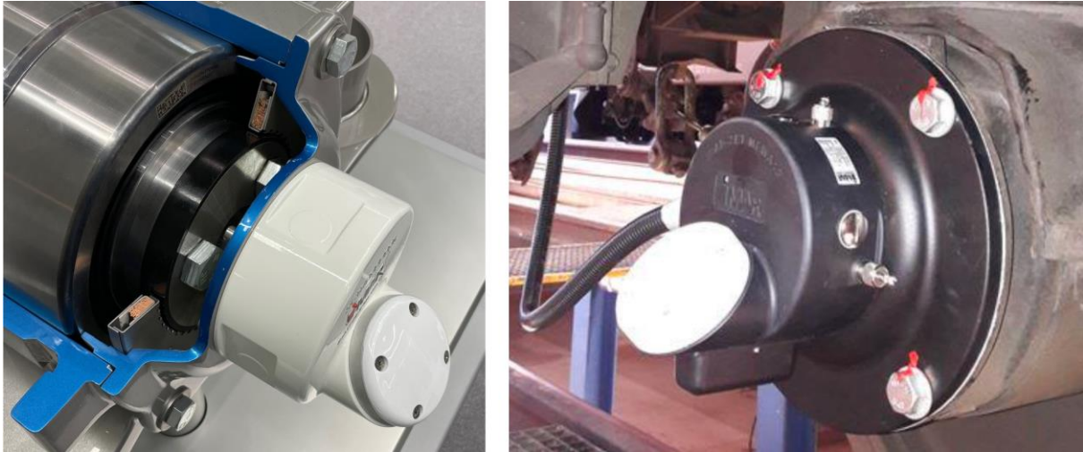
Figure 4: SmartRail 4.0, iZET-Rad prototypes: InnoTrans 2022 with Schaeffler axle generator (left), iRAD mounted on SBB MeWa12 axle (right)
